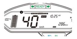
The current indication **O** displays the real-time current in the form of a status bar. You can roughly determine the current real-time current through the status bar When the status bar is full, the current is about 80Ah
