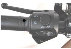
The headlight high/low beam **1** switch is on the left handle switch.
