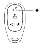
Use the remote controller's unlock key O to unlock the motorcycle
