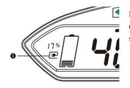
During cycling, when you brake the vehicle, the controller recovers the braking energy. At the same time the charging symbol **0** will light up.
