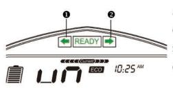
An arrow on the upper speedometer flashes green in the same direction as selected by the steering lamp switch. This remains flashing until the steering lamp request has been canceled.
