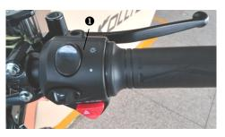
Flip the switch upward to ☆, open the Headlight. Flip the switch down to ●, open the Headlight.
