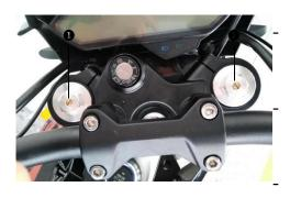
The hydraulic rebound damping system determines the performance of the front suspension when it bounces up. The adjusting bolt • is located at the upper end of the front suspension leg.
