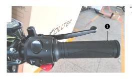
The throttle grip **0** is fitted on the right side of the handlebar.
