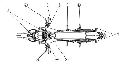
Front switch light 2 Front brake handle 3 Accelerating handle 4 Right handle switch
