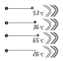
The system can display four temperatures, with "B" above the temperature display value indicating current battery temperature, "C" indicating current controller temperature, "M" indicating current motor temperature and no label indicating current external temperature.
