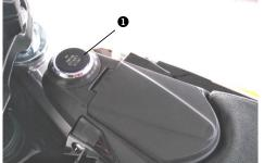
Start/stop button is used to start or stop the motorcycle.
