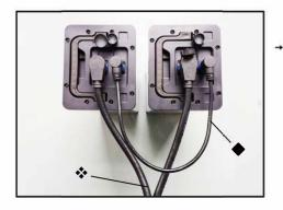
The figure on the left is the schematic diagram of double-battery connection. First connect the two batteries with the battery connecting line, and then connect the two batteries respectively to the connector of the main wire bundle.
