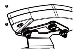
The adjustment button ② is located on the right back of speedometer ①. And it operates in two ways.
