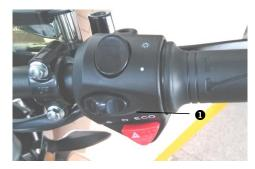
The driving mode switch **①** is on the right handle switch. Toggle between ECO, D(Dynamic), and S(Sport) modes. The ECO selection reduces the acceleration and top speed of the motorcycle but increases the amount of regeneration when the throttle is released. It is an ideal mode for when you want softer acceleration. This position is also good for newer riders and for extending range.
